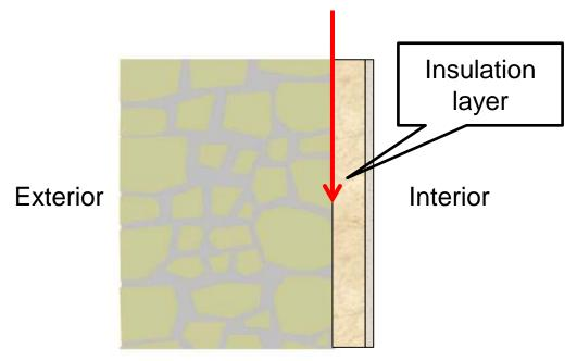
The simplest solution is to measure the Relative Humidity (& temperature) at the interface.
