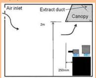
The canopy hood needs to be designed and operated to ensure the efficient removal of cooking fumes. It will need to be of a suitable size and have sufficient extraction to minimise fume spillage into the kitchen.
