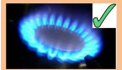
Most equipment now has inbuilt ignition and pilot light systems. However, if these fail or are not available then you may need to manually light using a taper or appropriate gas igniters.
