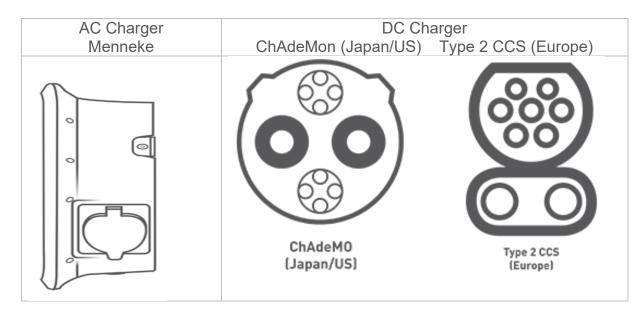
The difference between the two being the DC current directly charges the batteries in the electric vehicles, as opposed to AC chargers which utilise the rectifier in the vehicle to turn AC from the supply into DC to charge the battery. In most cases, the rectifier in the vehicle is limited to between 3 and 11 kW, using a single phase of AC power<sup>9</sup>.
