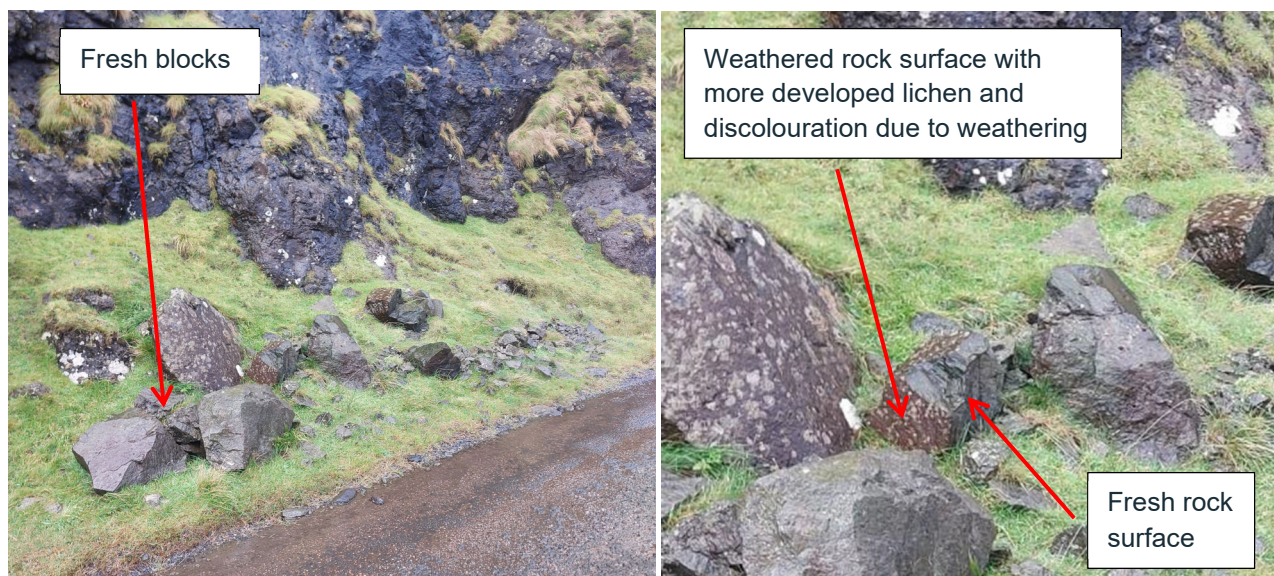
Figure 3-7 - (Left) Fresh rock blocks located immediately adjacent to the road, their positioning indicates that they may have been removed from the road by road users following failure. (Right) fresh surfaces visible on an otherwise weathered rock block indicating that the block may have been mobilised from the rock face, or impacted by another falling rock fairly recently
