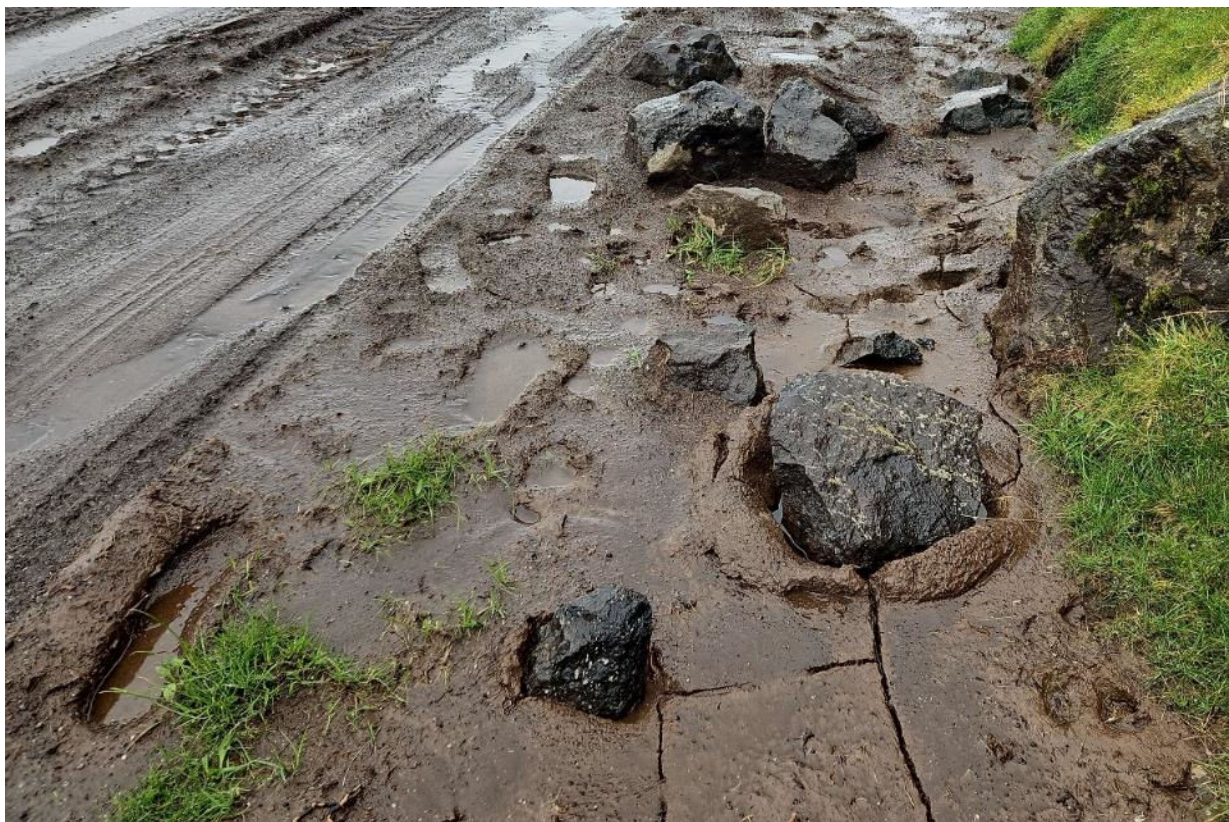
Figure 3-9 - Block that has displaced fine debris material, indicating that it mobilised after the debris was washed onto the road. Block is approximately 0.2 m across
