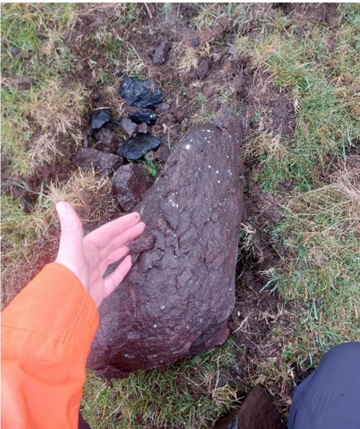
Figure 3-2 - Weathered basalt block (in impact crater) which the surface layer was able to be broken by hand, indicating a loss in strength
