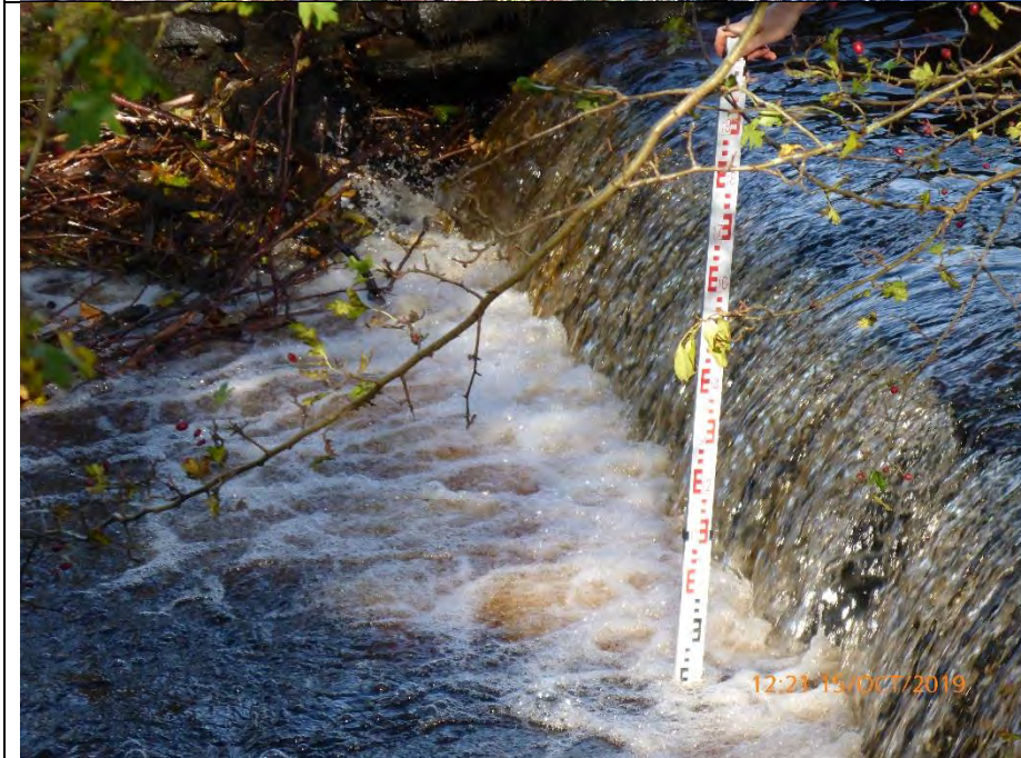
Figure 4: Close up of weir showing the depth of the weir pool and relative height of the weir.
