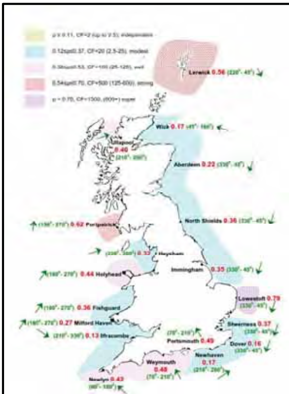
Figure 6-7: Correlation coefficient (p, wave height & sea level) Wave direction where dependence is highest.
