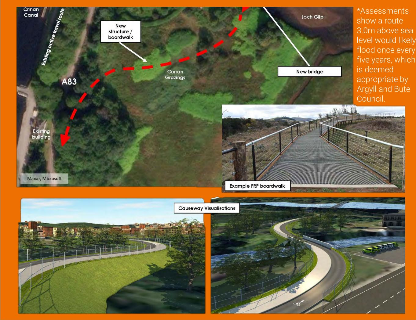
3.0m bidirectional cycle path (as specified by Cycling by Design).
