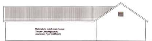
Pool House/Workshop West Elevation Scale 1:100 # A1
