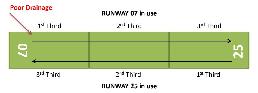
**NOTE**: If 2/3 of the Runway are not suitable for use by aircraft, the Airfield is likely to be closed. Glenforsa has a tradition of poor drainage at the 07 NW area and aircraft are advised to land on the high side (see arrow above).
